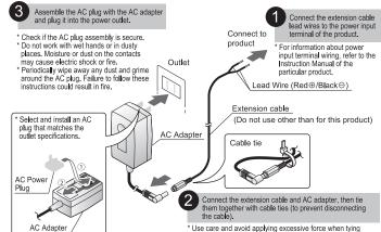
Use care and avoid applying excessive force when tying cables with cable ties.
