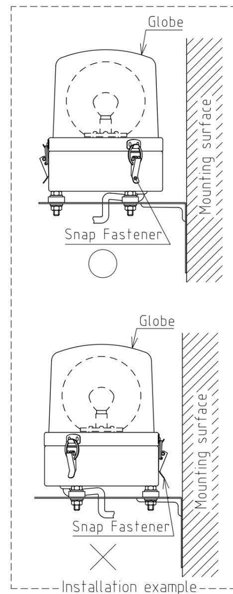
Material : SECC-P(Electro-galvanized Iron), t1.6
