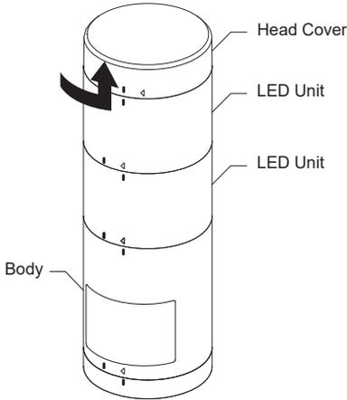
While holding the LED unit, turn the head cover counterclockwise until it unlocks, then pull it upwards to remove.
