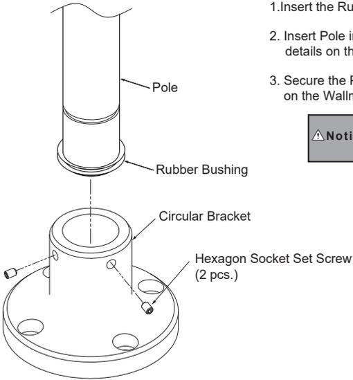
1. Insert the Rubber Bushing into the pole.
