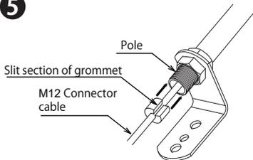
Insert the M12 connector cable through the slit in the grommet and insert the grommet into the pole.
