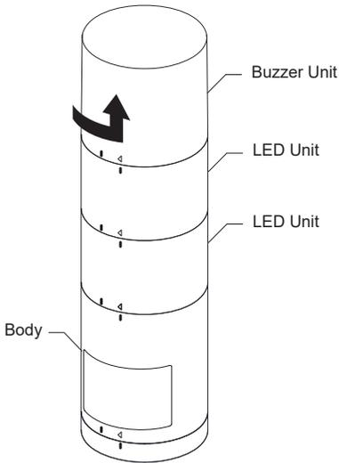
While holding LED unit, turn the buzzer unit counterclockwise, until it unlocks, then pull it upwards to remove it.
