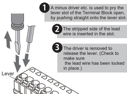
**1** A minus driver etc. is used to pry the lever slot of the Terminal Block open, by pushing straight onto the lever slot.
