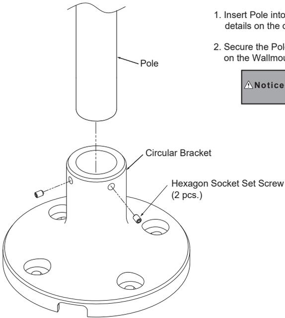
1. Insert Pole into the Circular Bracket. See the figure on the left for details on the direction of insertion.
