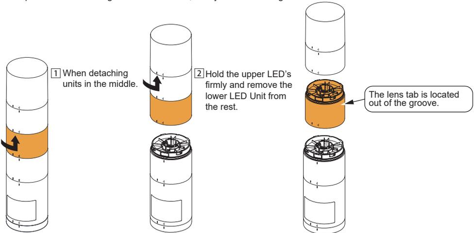
If the LED Unit can't be attached, try the procedure below.
