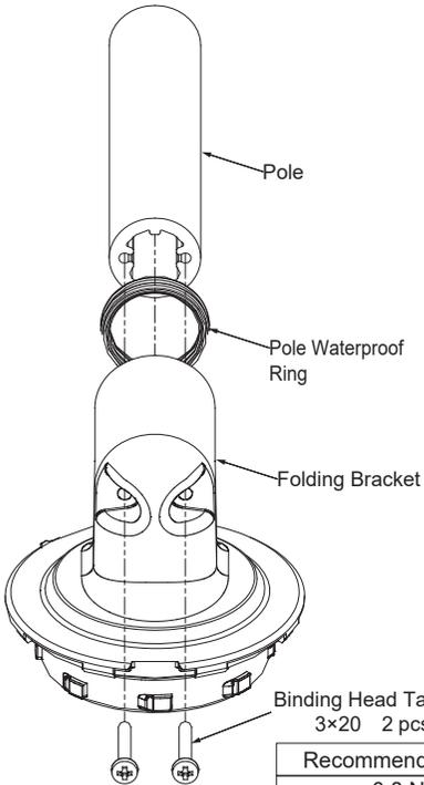
1. Install the Pole Waterproof Ring in the Folding Bracket. Check that the 2 ribs are on the outside.
