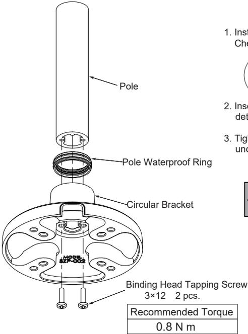
1. Install the Pole Waterproof Ring in the Circular Bracket. Check that the 2 ribs are on the outside.
