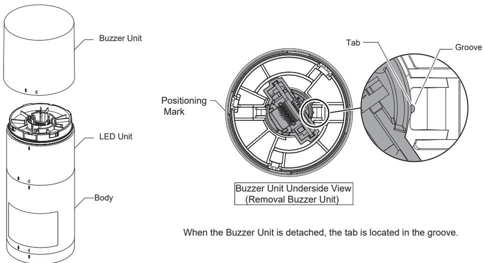
When the Buzzer Unit is detached, the tab is located in the groove.
