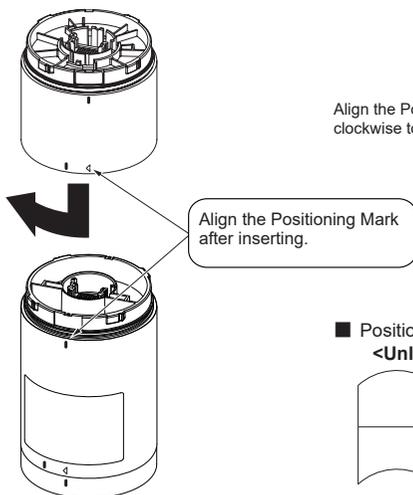
Align the Positioning Mark after insertion, then turn the unit clockwise to lock it.
