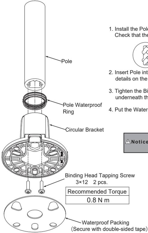
1. Install the Pole Waterproof Ring in the Circular Bracket. Check that the 2 ribs are on the outside.
