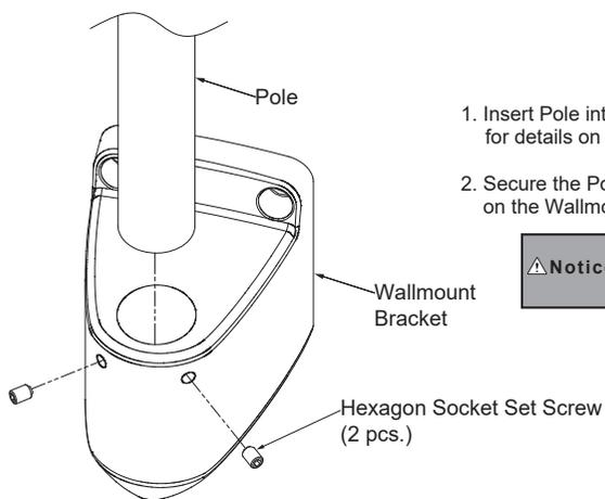
1. Insert Pole into the Wallmount Bracket. See the figure on the left for details on the direction of insertion.
