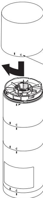
Align the Positioning Mark after insertion, then turn the unit clockwise to lock it.
