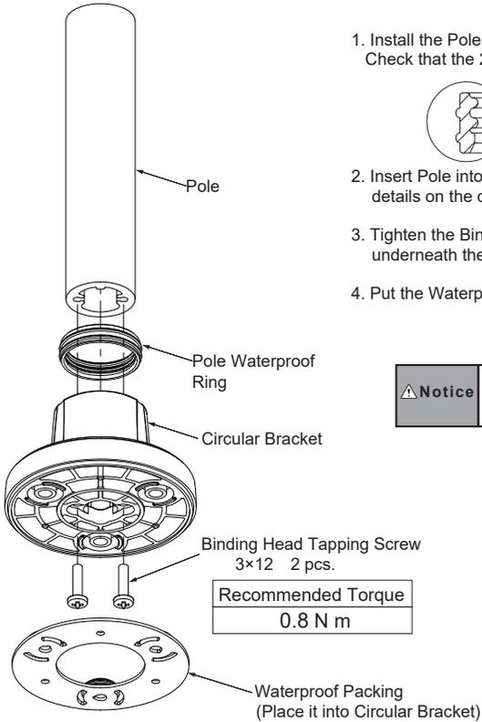
1. Install the Pole Waterproof Ring in the Circular Bracket. Check that the 2 ribs are on the outside.
