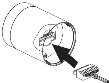
Attach the terminal block connector to the body unit after wiring.
