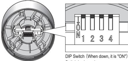
DIP Switch (When down, it is "ON")
