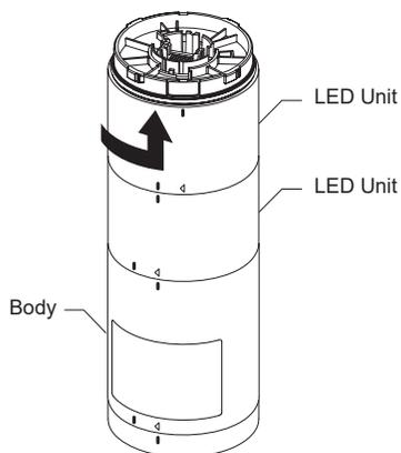
While holding LED unit, turn the LED unit counterclockwise, until it unlocks, then pull it upwards to remove.
