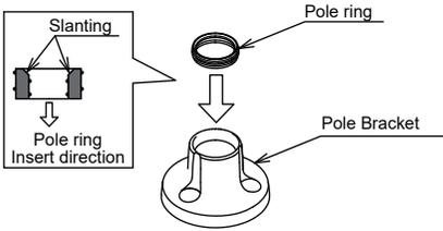
2. Assemble the pole and Pole Bracket.
