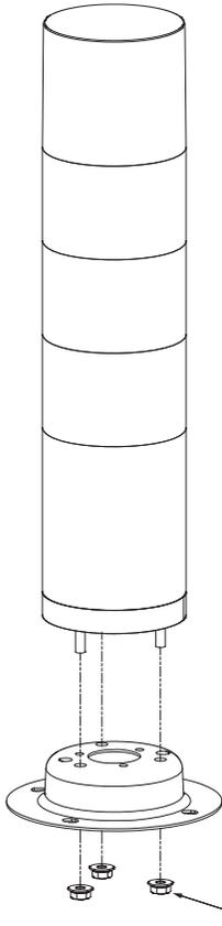
1. Insert the mounting screws of the product into the Circular Bracket. See the figure on the left for details on the direction of insertion.
