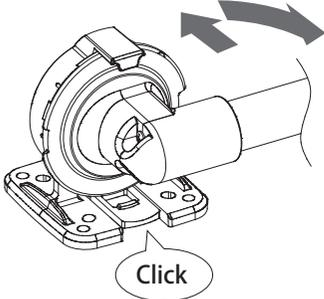
Pushed down in a clockwise direction
