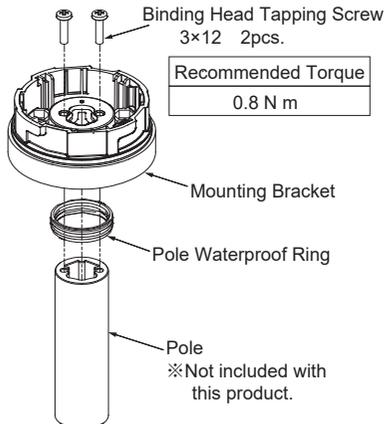
1. Be sure to remove the waterproof packing from the Mounting Bracket.
