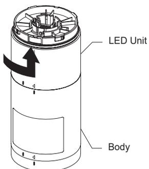
While holding the body, turn the LED unit counterclockwise, until it unlocks, then pull it upwards to remove.
