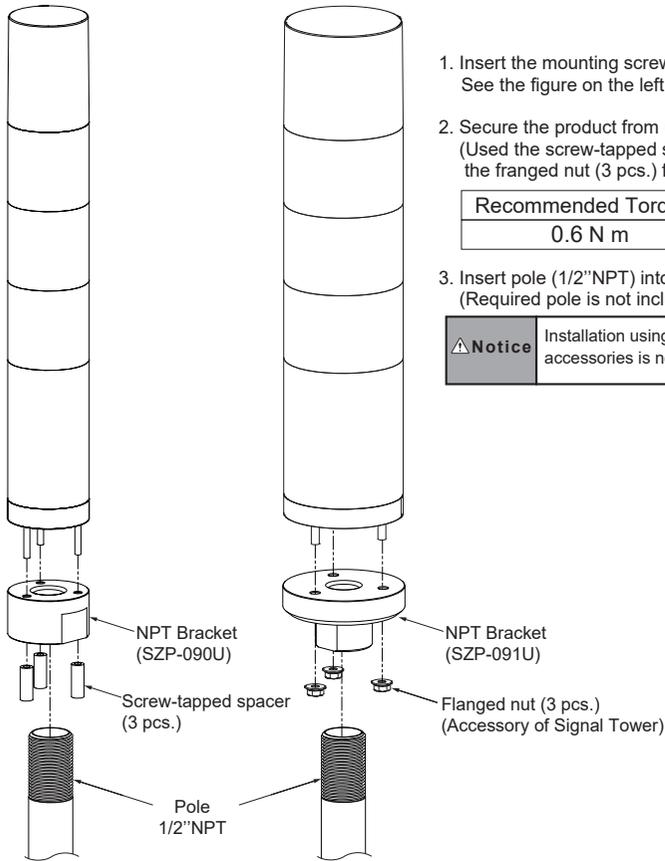
1. Insert the mounting screws of the product into the NPT Bracket.
