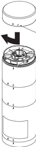
Align the Positioning Mark after insertion, then turn the unit clockwise to lock it.
