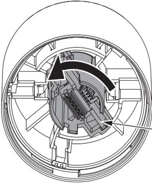
Turn the internal part of the Buzzer Unit counterclockwise until the tab fits in the groove.
