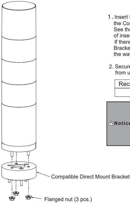
1. Insert the mounting screws of the product into the Compatible Direct Mount Bracket. See the figure on the left for details on the direction of insertion.
