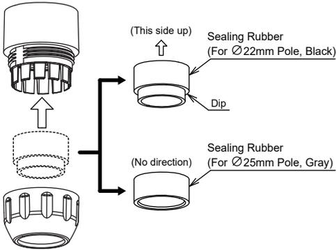
3. Slide the Pole through Upper Bracket B and insert the top end of the Pole into the Sealing Rubber.
