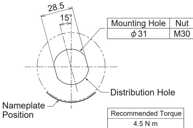
■ **LR6**-**W4/W5/W8** **WC** Installation Figure (1/2" NPT Installation Figure)
