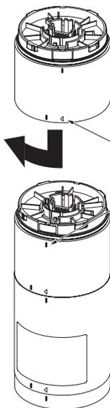
Align the Positioning Mark after insertion, then turn the unit clockwise to lock it.
