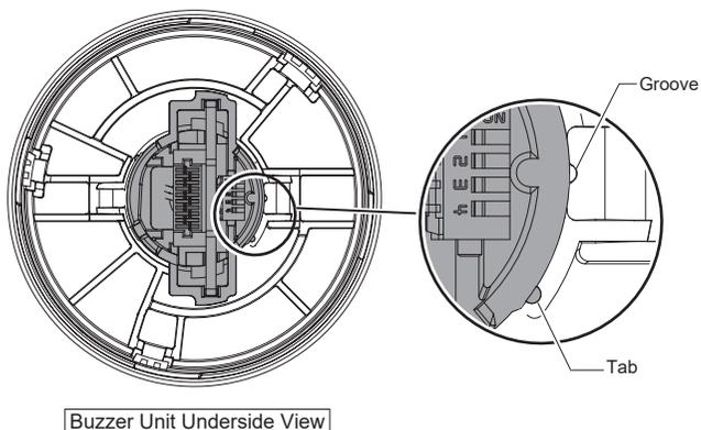
If the Buzzer Unit can't be attached, try the procedure below.
