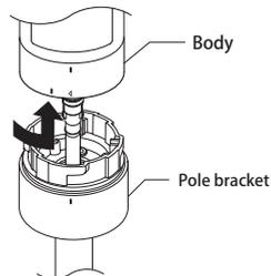
Remove the pole bracket from the body and remove the M12 connector cable.
