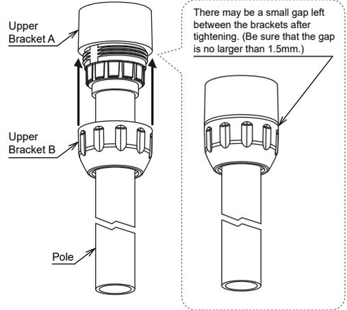
5. Pass the M12 Connector Cable through the Upper Bracket and Pole, connect the M12 Connector Cable to the LR4-WC (1), then tighten the LR4-WC to the Upper Bracket (2).
