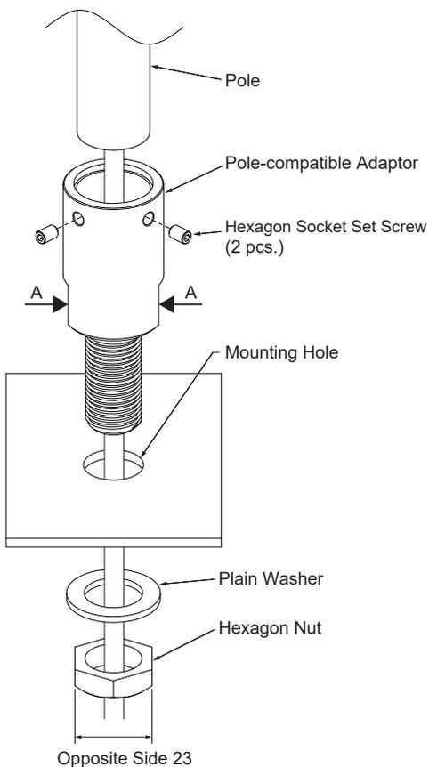
1. Run the wiring through the the Pole-compatible Adaptor. Insert the Pole into the Pole-compatible Adaptor.
