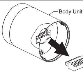
Remove the connector from the body unit before wiring.
