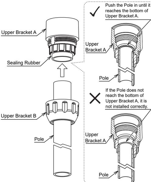
4. Tighten Upper Bracket B into Upper Bracket A.
