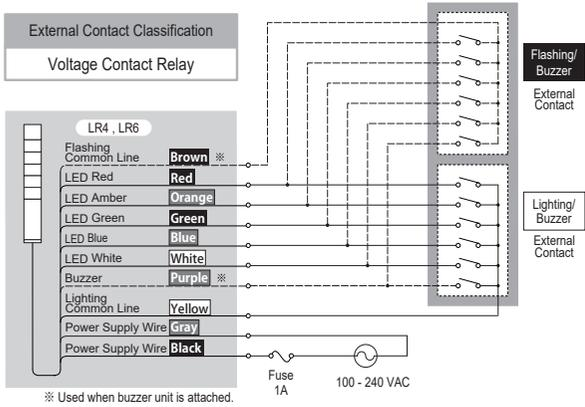
Only apply voltage to Power Supply Wires.
