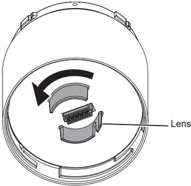
Turn the internal lens of the LED Unit counterlockwise until the tab fits in the groove.
